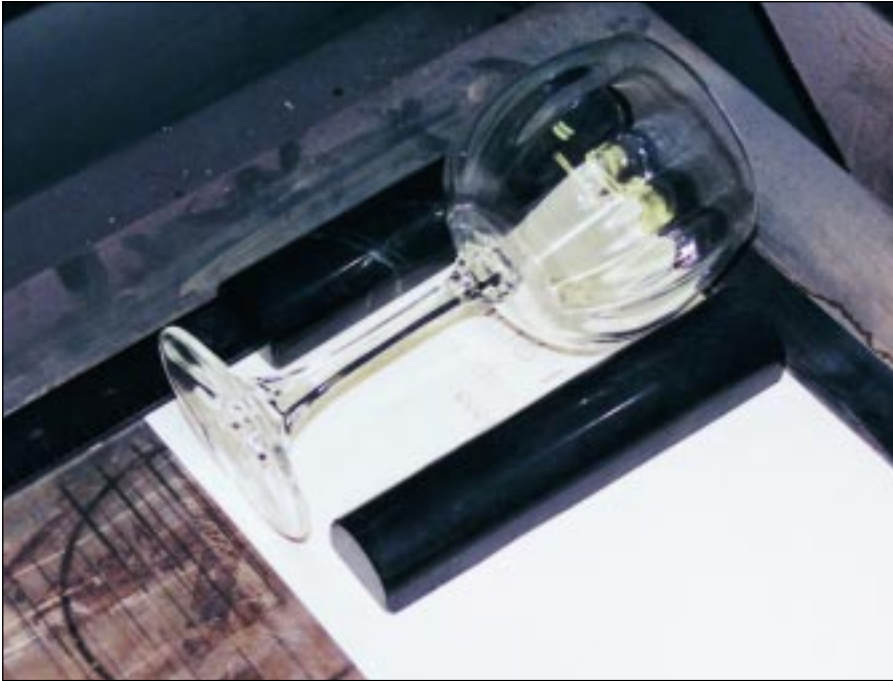
Wine glass being prepared for engraving. Note the two marble bars used to hold the glass securely in place for engraving.
