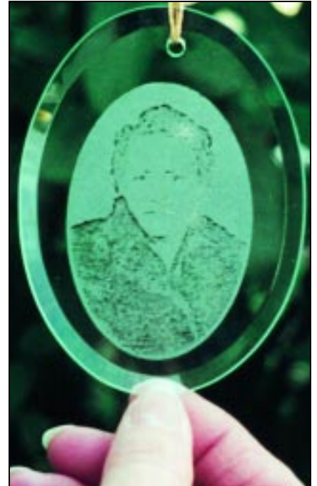
Even photographs can be engraved in glass. Using a special photoengraving program, this was easily engraved in a single pass.
