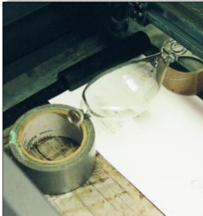
Here, an extremely odd-shaped piece of hand-blown glass is being engraved. Almost anything can be used to create simple jigs to hold odd-shaped items in a laser. Here, two different-sized rolls of tape form a perfect platform to hold this glass weather indicator.
