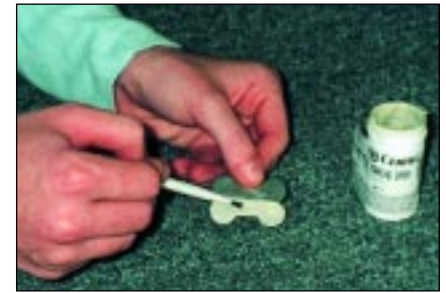
Certec should be applied with a small airbrush but in the absence of compressed air, it can be brushed on with a small brush for dog tags and other small items or a foam brush for larger items. A smooth even coat is necessary for good result.
