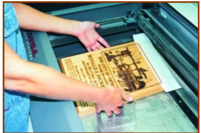
(Below) Prevention is always the best cure. Here, an alder plaque is being removed from the engraver. Note the protective tape at the top. Although it proved not to be necessary in this case, it is necessary in many cases when heavy or deep lines are cut into wood.
