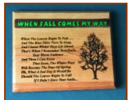
Here an alder plaque shows off its natural contrast while the top is highlighted by green laser foil on raised letters. This is a simple process but does demand some planning. Notice a very bold font was selected for use with the foil letters.
