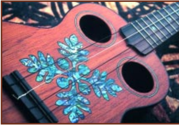
Fantastic inlays can be created with lasers. Here, a guitar has been engraved and inlaid with seashell material. The process is fast, simple and demands a big return.
