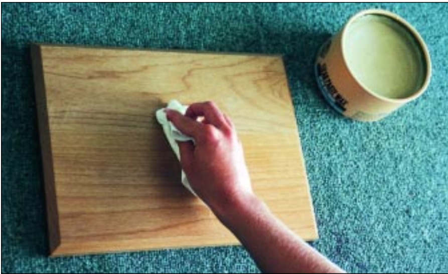
Preparing the wood for engraving is often just as important as the engraving itself. Here, a wood plaque is being waxed using a good paste floor wax.
