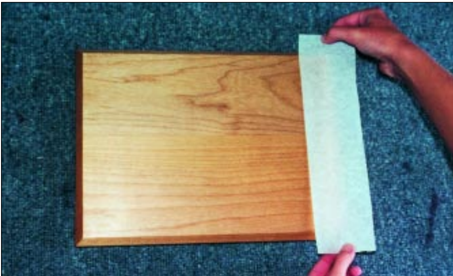
Sometimes, wax alone isn't enough to protect the wood. Here, some paper transfer tape is being added to the top of a plaque to protect it from damage while a very heavy engraved area is being cut.
