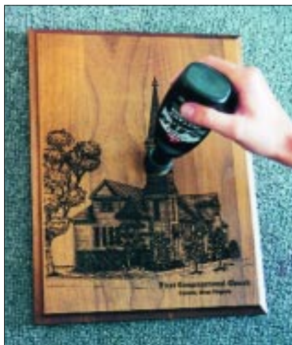
One of the best and most commonly used blackening agents for wood engraving is liquid shoe polish. Just dab it on, smear it around a little and wipe it off.
