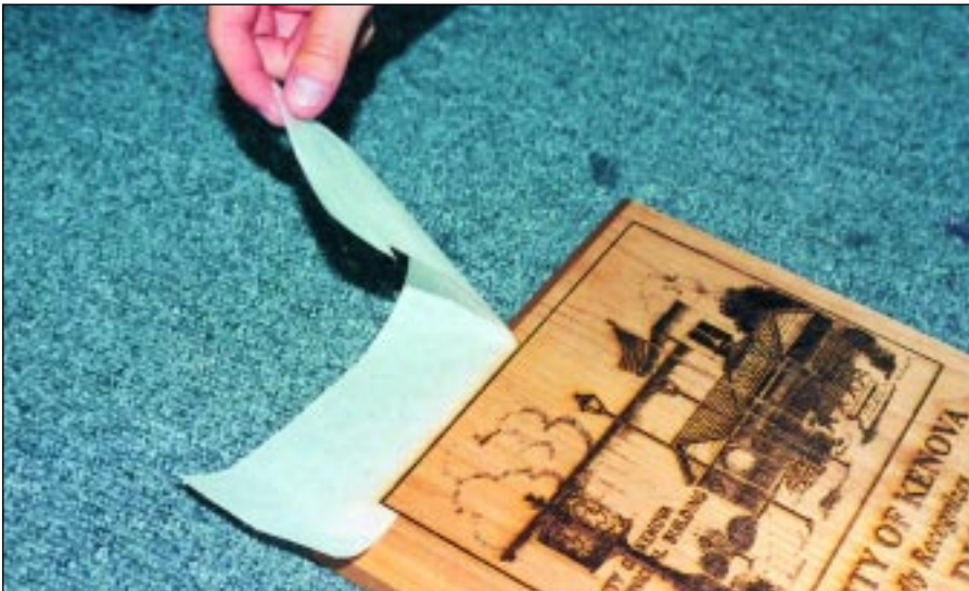
Here, the protective tape is removed to reveal an engraved area with no damage to the surrounding wood.
