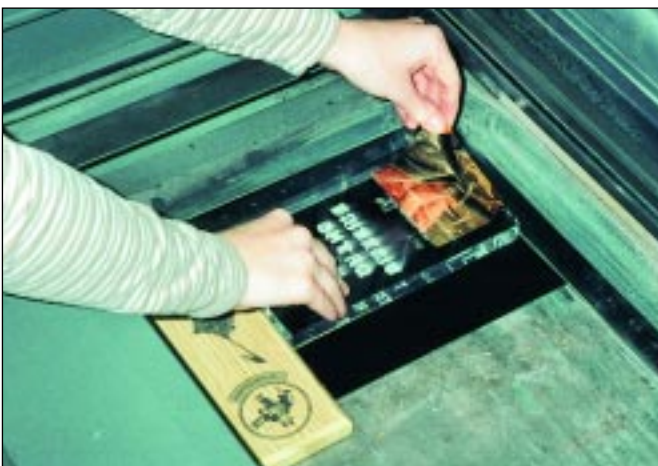
The excess of the gold foil being removed after being lasered. Remove slowly and carefully to avoid damage to the finished logo.
