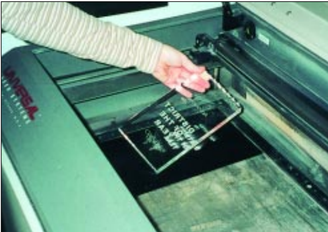
The acrylic award after the reverse side has been engraved. It will now be turned over and prepared for the foil applique.
