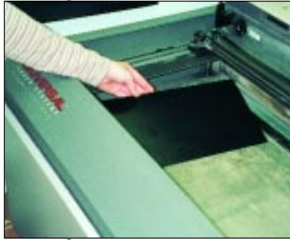
Placing a sheet of aluminum in the engraver. This will be used for making a safety engraving.
