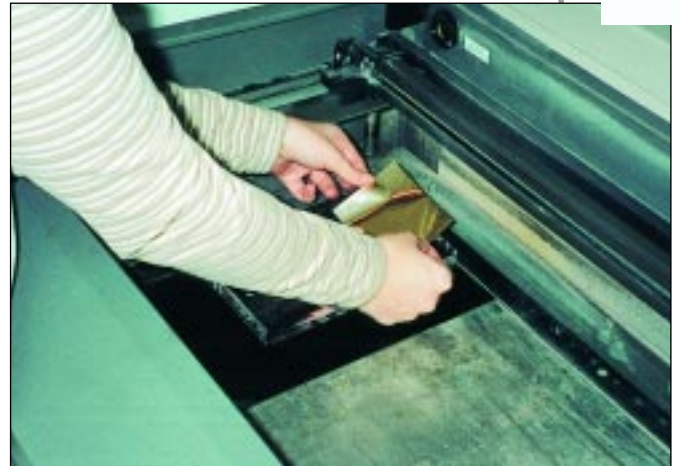
The self-adhesive foil being applied to the acrylic.
