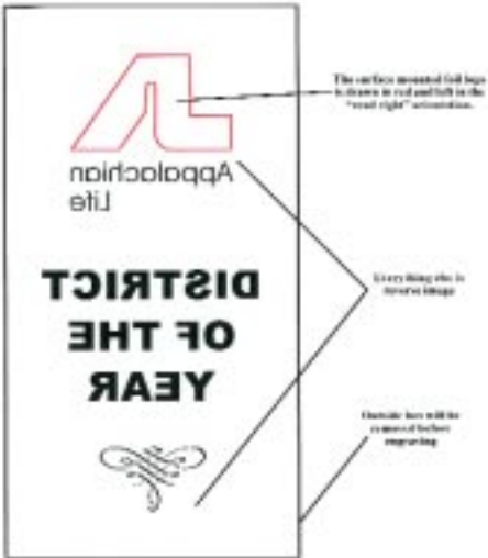
This is what the layout will look like on the computer screen. Note the logo is read right while everything else is reversed.
